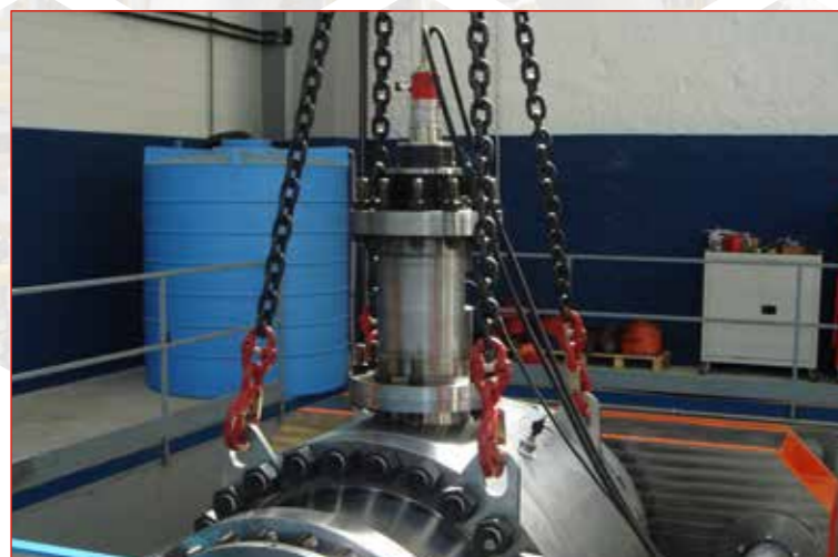
TRANSDUCER Measuring the applied torque of the valve Transducer is connected either to a display instrument (for real-time reading of torque) or a control panel (for torque reading and control features)
